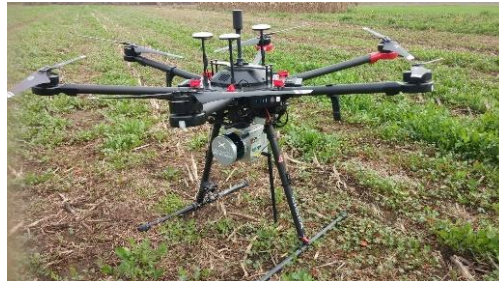
Figure 4 – The LiDAR data acquisition system
